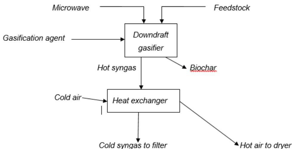
Figure 2. A schematic of the Endeavour Energia S. r. L's Endeavour Microwave Gasification Technology. Supplied by the developer in response to a questionnaire [2].
