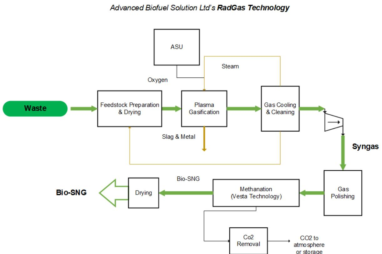
Figure 9. A schematic for the Advanced Biofuel Solution Ltd's RadGas technology as implemented in the Swindon plant. Adapted from a 2016 presentation at a Global Syngas Forum conference by representatives of Advanced Plasma Power (the then project developer) and Amec Foster Wheeler (the methanation system supplier) [7]
