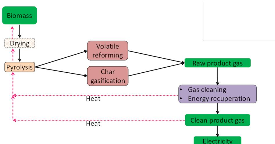
Figure 1. A schematic of the Renergi Pty Ltd's Advanced Biomass Gasification Technology. Based on the schematic diagram provided in [3]
