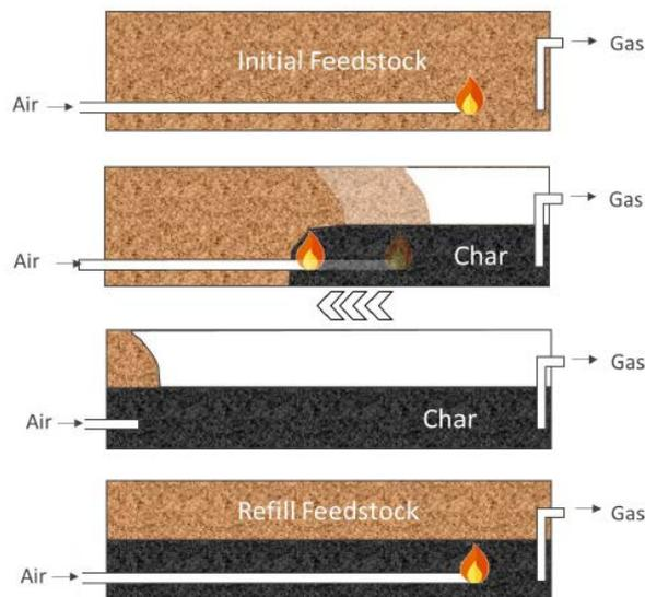
Figure 5. Schematic showing oxidant injection retraction and subsequent gasification front sweeping through the feedstock. Provided by the developer [4]
