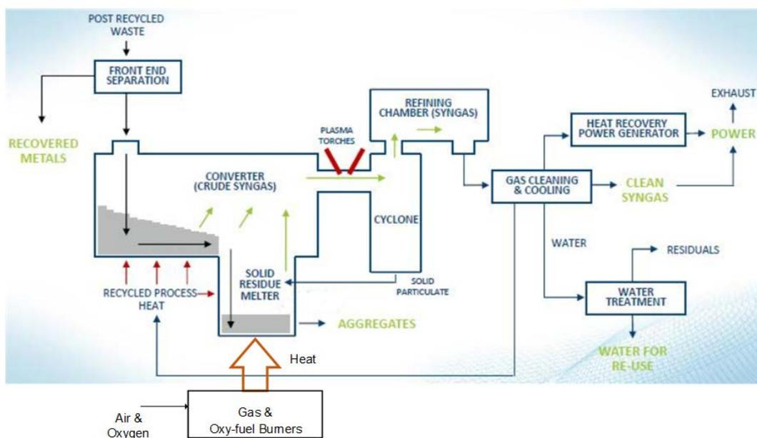
*Figure 8. Integrated Conversion & Refining System, taken from [2] and adapted to represent the present heating arrangements for the solid residue melter*
