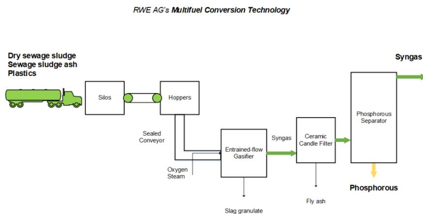
Figure 7. A schematic for the MFC technology-based Niederaussem pilot. Adapted from a presentation by one of the partners in the ITZ-CC project (pilot testing of the MFC technology) [5]
