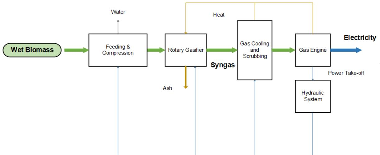
Figure 10. A simplified schematic for SUNY Cobleskill's Inclined Indirect Flaming Pyrolysis Rotary Gasifier based on [1, 2]
