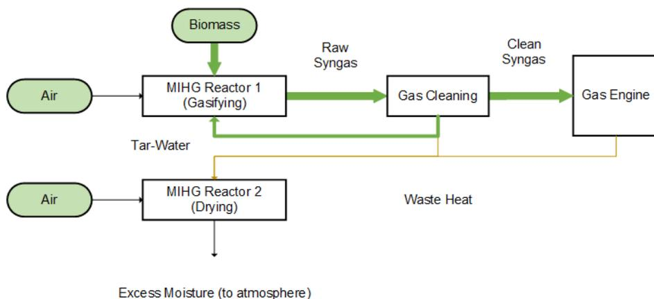
Figure 6. A schematic for the MIHG technology in a dual-reactor biomass-to-electricity application. Adapted from [1]
