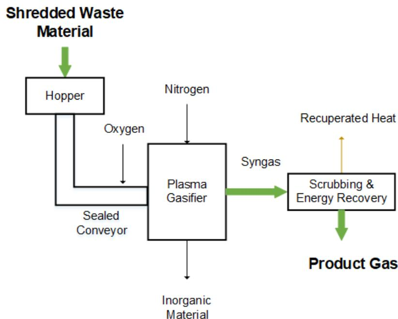
Figure 3. A schematic of Cogent Energy Systems' Heliostorm™ Gasification technology. Adapted from a 2019 presentation of the concept [2]
