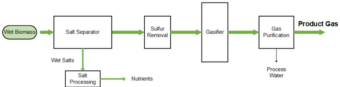
Figure 11. A simplified schematic for TreaTech's Hydrothermal Gasification System
