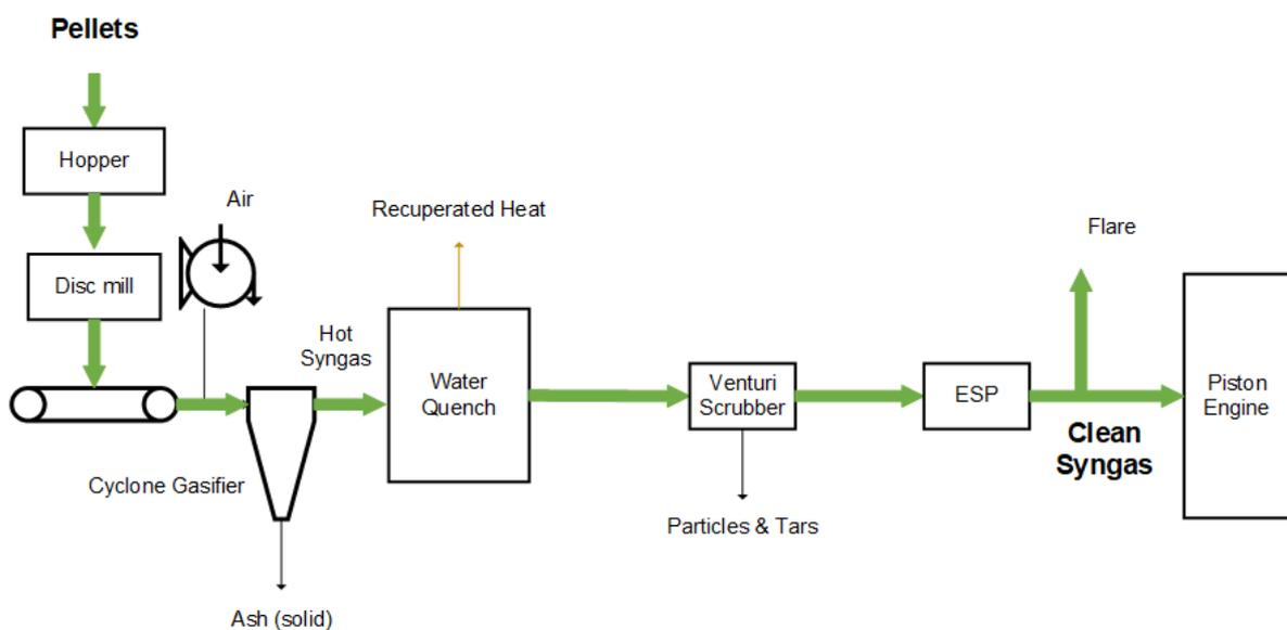
Figure 4. A schematic for MEVA Energy AB's technology. Adapted in modified form from [4]
